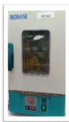
20g of sample at 65°C 24 hours in hot air oven
