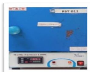
5g of sauce sample into the crucible at 550°C
