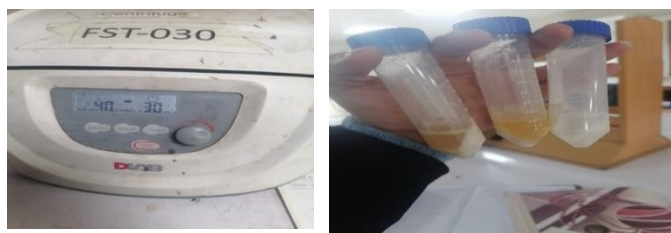
Figure 2: Determination of water absorption capacity of flour of T 0 , T 1 , and T 2 performed in Lab II at the University of Central Punjab, Lahore
