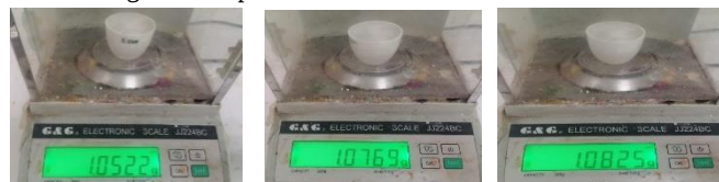
Figure 5: Determination of ash content of products T 0 , T 1 , and T 2 performed in Lab II at the University of Central Punjab, Lahore
